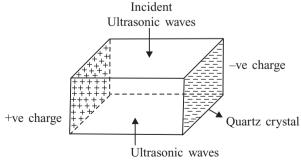
Fig. 1.4 Schematic representation of piezoelectric detector
