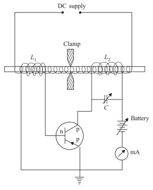
Fig. 1.2 Circuit diagram of magnetostriction method
