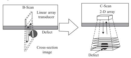
Figure 1.17 shows the difference between a B-scan and a C-scan.
