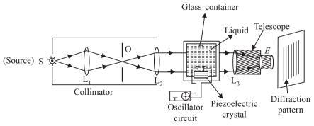
Fig. 1.6 Schematic diagram of acoustic grating
