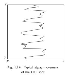
The reflected echo received by the probe forms the Z-axis input for the CRT. Pulsed output from the rate generator is also fed to the time-base generator whose output is given to the X-plates of the CRT. The signal applied between the X-plates is used to deflect the electron beam of the CRT. The vertical deflecting plates (Y-plates) are fed the output of a low-frequency time-base generator. This input makes a bright spot on the screen of the CRT that executes vertical motion at a slow speed.
