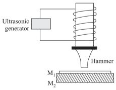
Fig. 1.8 Ultrasonic welding system
