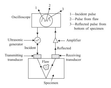
Fig. I.I I Ultrasonic flaw detection system
