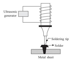
Fig. 1.9 Ultrasonic soldering system
