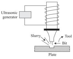
Fig. 1.7 Ultrasonic drilling system
