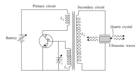
Fig. 1.3 Piezoelectric oscillator circuit
