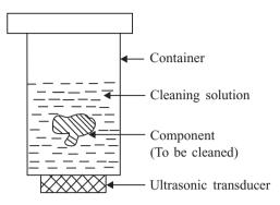
Fig. 1.10 Ultrasonic cleaning system
