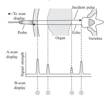
Figure 1.15 shows schematic representation of A-scan and B-scan displays.
