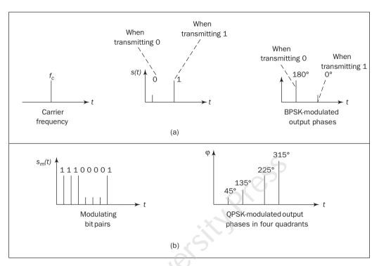
**Fig. 1.7** (a) BPSK signal for transmitting the bits (01) (b) QPSK signal for transmitting four bit pairs 11100001
