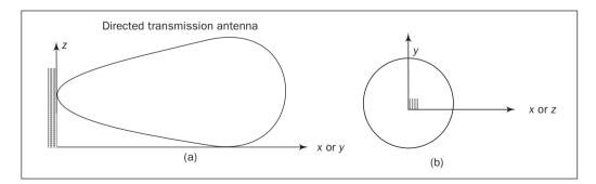
**Fig. 1.4** (a) Radiation pattern along the z-y and z-x planes in a directed transmission case antenna (e.g., between a base station and mobile phone) (b) Radiation pattern of the same antenna along the x-y plane
