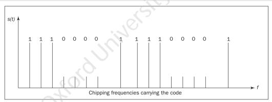
**Fig. 1.8** Carrier signal frequencies in spread spectrum when 1110000111100001 coded 16 chipping frequencies XORed with the symbol S = 0 () during a chipping interval of transmission
