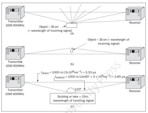
**Fig. 1.5** (a) Scattering of signal, (b) Diffraction of signal, and (c) Reflected and direct signals from a 900 MHz transmitter and calculation of delay
