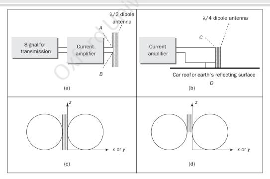
**Fig. 1.3** (a)  $\lambda/2$  dipole antenna, (b)  $\lambda/4$  dipole antenna, (c) Radiation pattern in *z*-*y* and *x*-*z* planes for  $\lambda/2$  dipole, and (d) Radiation pattern in *y*-*z* and *x*-*z* planes for  $\lambda/4$  dipole of wavelength  $\lambda$ . It is also called a *dipole antenna* because at any given instant, at both the ends A and B, the signals are 180° out of phase.
