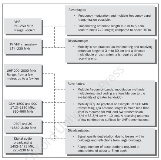
**Fig. 1.2** Wireless transmission in VHF and UHF ranges: frequencies and properties will be reduced and different, depending on the dielectric constant).
