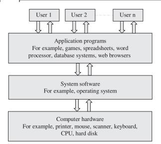
Figure 1.49Relationship among hardware, system<br/>software, and application software
