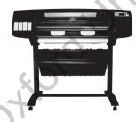
plotters worldwide. There are **Figure 1.41** Plotter two different types of plotters—drum and flatbed (refer Figure 1.41).
