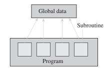
Figure 1.63 Structure of a procedural program
