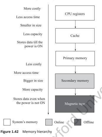
CPU first checks whether the data or instruction is available in cache memory. If it is not present, the CPU reads the data or instructions from the main memory into the processor registers. The CPU also copies it into the cache memory. When the same piece of data/instruction is needed, the CPU reads it from the cache memory instead of the main memory.
