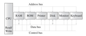
Figure 1.17 Buses with a computer system
