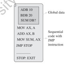
Figure 1.62 Structure of a monolithic program
