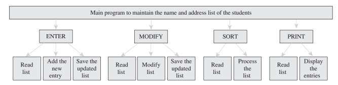
Figure 1.66 Layered program structure
