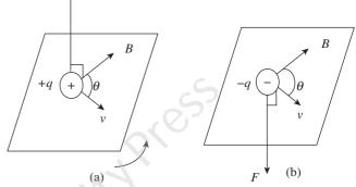
**Fig. 1.12** Right hand rule to determine the direction of Lorentz force – (a) On a positive charge (b) On a negative charge
