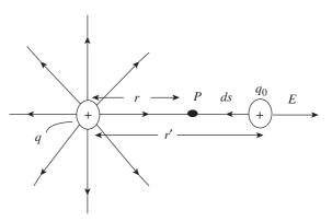
**Fig. 1.10** The positive point charge *q* produces an electric field *E* and an electric potential *V* at point *P*
