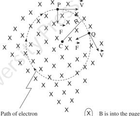
Fig. 1.18 Force exerted by a uniform magnetic field on a moving charged particle (in this case, an electron) produces a circular path
