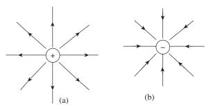
Fig. 1.3 Electric field lines (a) near a single positive point charge (b) near a single negative point charge
