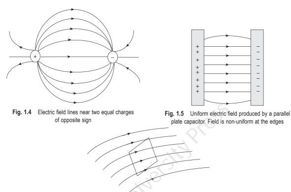
Fig. 1.6 Conventional representation of electric field intensity by the number of lines of force passing perpendicularly through a unit area
