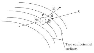
**Fig. 1.11** A test charge  $q_0$  moves distance *ds* from one equipotential surface to another. The displacement ds makes an angle  $\theta$  with the direction of the electric field  $\vec{E}$
