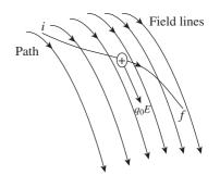
**Fig. 1.9** A test charge  $q_0$  moves from point *i* to point *f* along the path shown in a non-uniform electric field. During a displacement *ds*, an electrostatic force  $q_0E$  acts on the test charge. This force points in the direction of the field line at the location of the test charge
