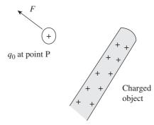
**Fig. 1.1** A positive test charge  $q_0$  placed at point P near a charged object
