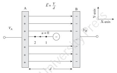
Fig. 1.13 Motion of electron in uniform longitudinal electric field
