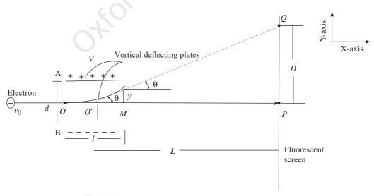
Fig. 1.14 Electron motion in transverse uniform electric field
