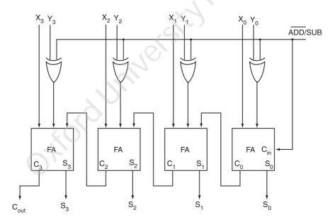
Fig. 5.15 4-bit parallel adder/subtractor
