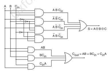
Fig. 5.5 Full-adder using basic gates
