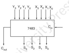
(a) Logic symbol of IC 7483-4-bit parallel binary adder
