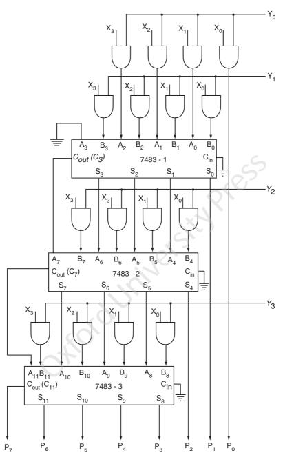
Fig. 5.25 4-bit parallel multiplier
