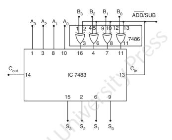
Fig. E5.1 4-bit parallel binary adder/subtractor using IC 7483
