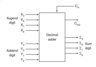
Fig. 5.20 Block diagram of a BCD adder
