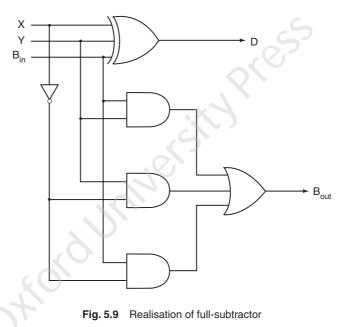
One can notice that the equation for D is the same as the sum output for a full-adder, and the borrow output  $B_{out}$  resembles the carry output for full-adder except that one of the inputs is complemented. From these similarities, it is possible to convert a full-adder into a full-subtractor by merely complementing that input prior to its application to the input of gates which form the borrow output.
