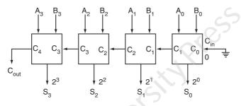
Fig. 5.10 4-bit binary parallel adder
