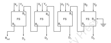
Fig. 5.12 4-bit parallel binary subtractor
