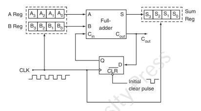
Fig. 5.17 4-bit serial adder
