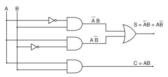
Fig. 5.2 Half-adder using basic AND, OR and NOT gates
