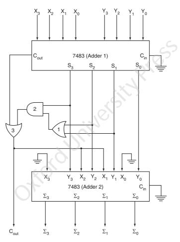
Fig. 5.23 BCD adder using 7483 ICs
