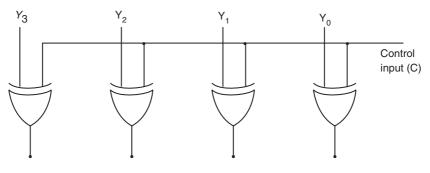
Fig. 5.14 Controlled inverter
