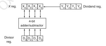
Fig. 5.27 Block diagram of a 4-bit binary divider
