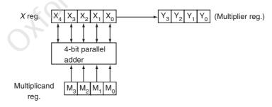
Fig. 5.24 4-bit binary multiplier using shift method
