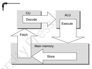
Figure 1.6 A simplified view of an instruction cycle
