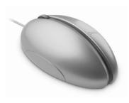
purpose of selecting or activating objects on graphical interface provided by the operating system or the software currently being executed and executing various tasks. It has two or three buttons for clicking. The mouse tracks the motion of the mouse pointer and senses the clicks and sends them to the computer so it can respond appropriately.
