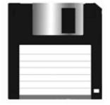
and can store 1.44 MB of data. Earlier PCs sometimes used 5½ inch disks. The disks store information and can be used to exchange information between computers. The floppy disk drive stores data on and retrieves it from the magnetic material of the disk, which is in the form of a disk. It has two motors one that rotates the disk media and the other that moves two read-write heads, each on either surface of the disk, forward floppy disk drive or backward.
