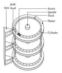
Figure 1.3 Schematic diagram of a hard disk
