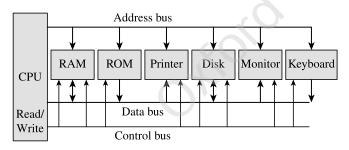
Figure 1.5 Buses with a computer system
