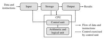
Figure 1.2 Block diagram of a computer
