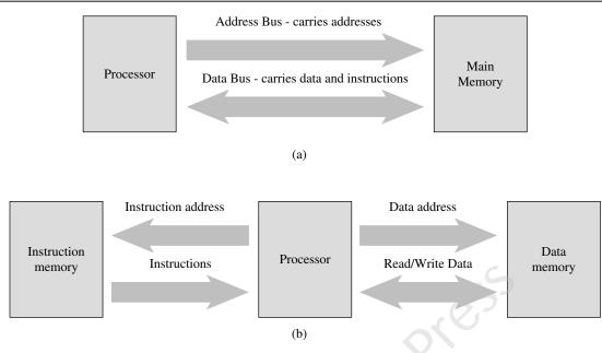
Figure 1.10 Von Neumann architecture (a) Shared memory for instructions and data (b) Separate memories for instructions and data
